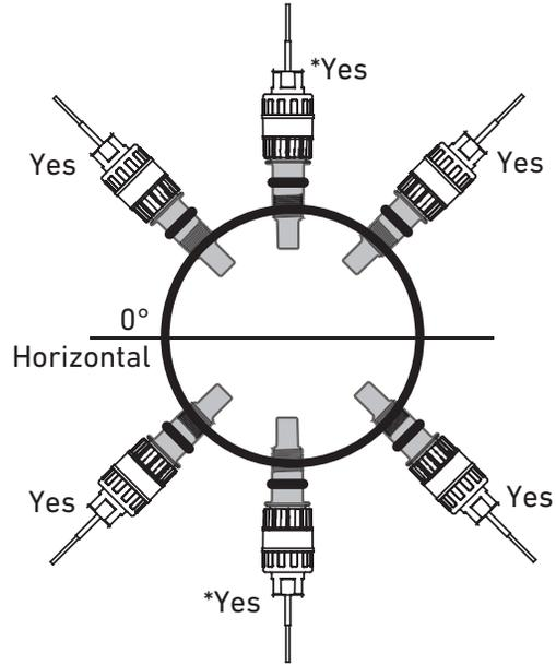
When mounting in standard threaded fittings the electrode must be mounted horizontally to 60 degrees below horizontal position only.
