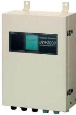
UVH-2000 is flowmeter constituted with velocity meter and level gauge to measure flows of sewage, wastewater, industrial effluent and other effluents contain fine particles, sludge or fine bubbles through pipes or open channels with free water surface.
